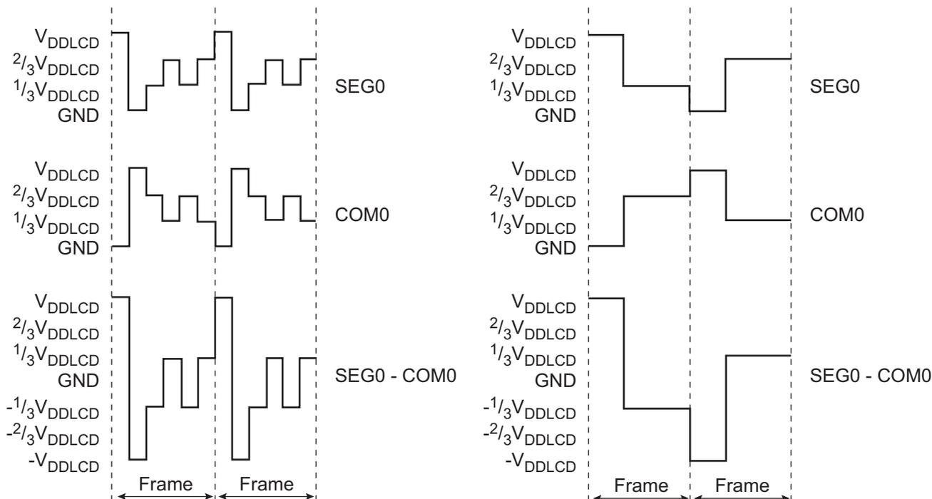
**Note:** Refer to the LCD specification to verify that low power waveforms are supported.
