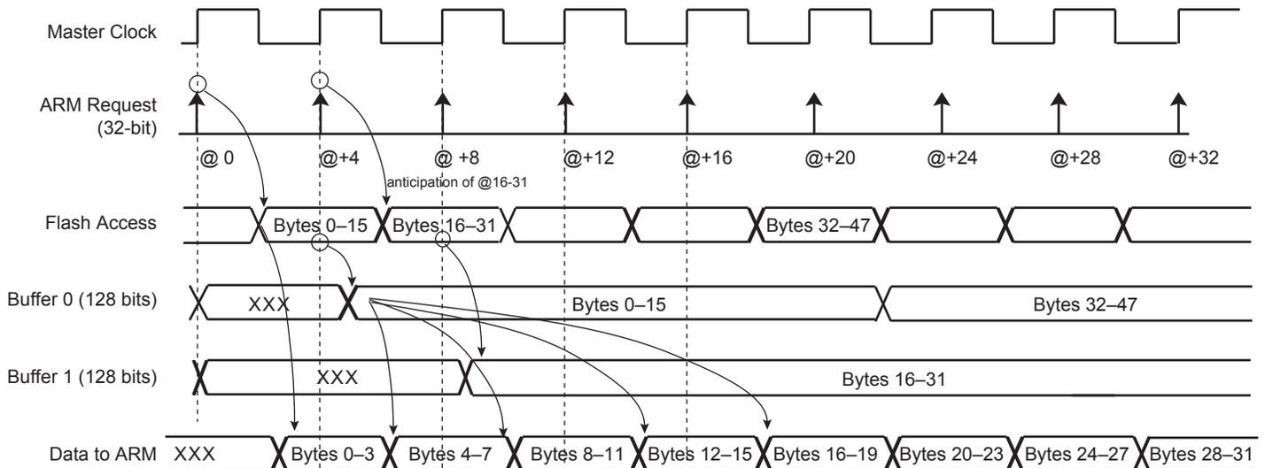
**Note:** When FWS is equal to 0, all the accesses are performed in a single-cycle access.
