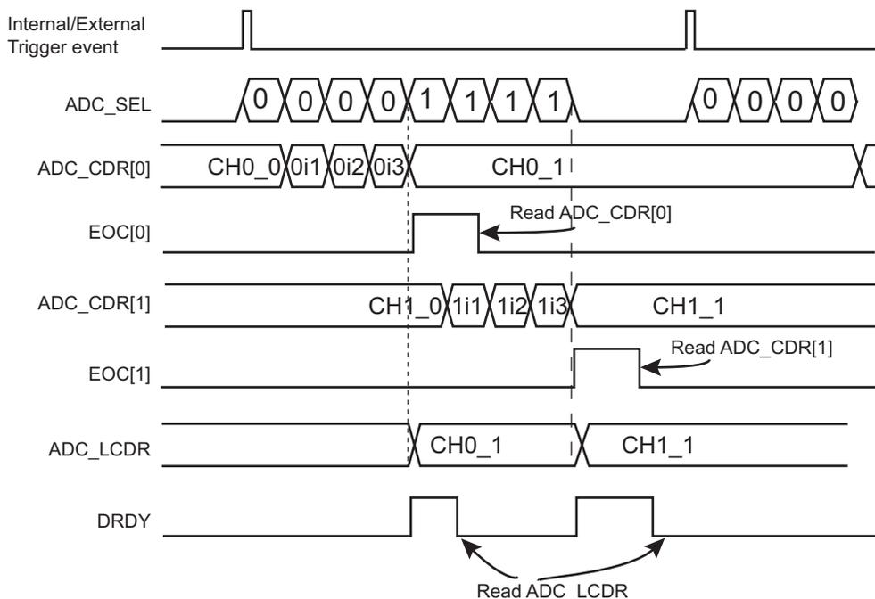
Notes: ADC\_SEL: Command to the ADC cell
