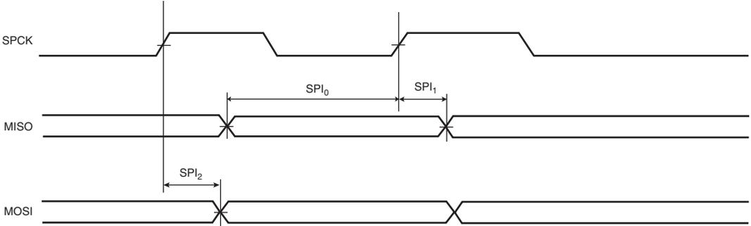
**Figure 46-5: SPI Master Mode with (CPOL = 0 and NCPHA=1) or (CPOL=1 and NCPHA= 0)**
