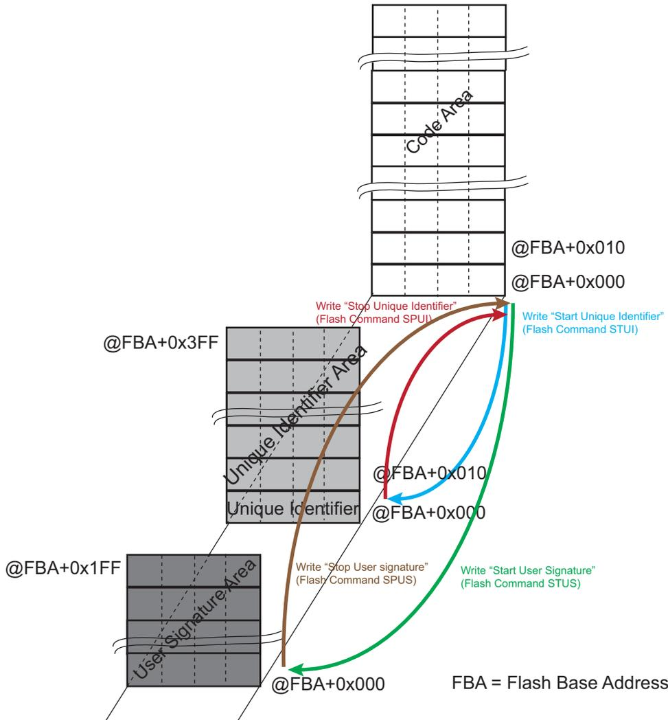
Figure 22-2: Organization of Embedded Dual-plane Flash for Code
