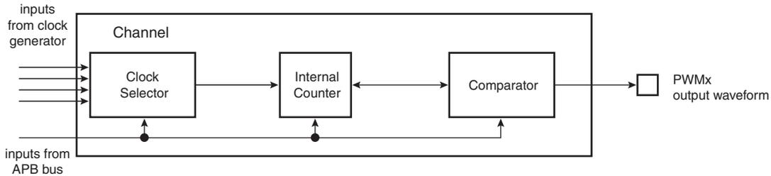
Each of the four channels is composed of three blocks:
