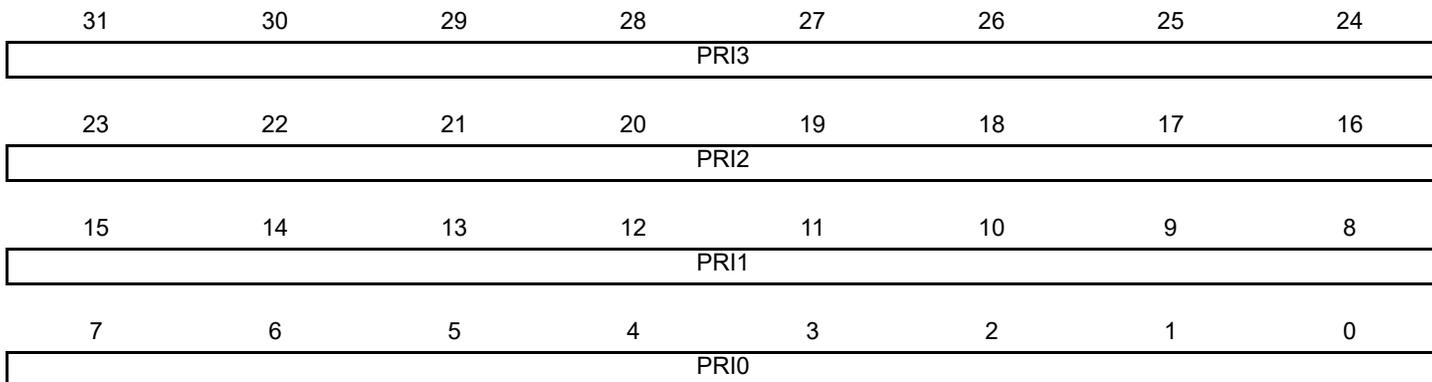
The NVIC\_IPR0–NVIC\_IPR10 registers provide a 8-bit priority field for each interrupt. These registers are byte-accessible. Each register holds four priority fields that map up to four elements in the CMSIS interrupt priority array IP[0] to IP[40].
