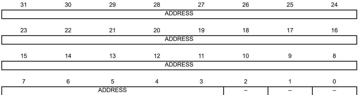
The FPCAR holds the location of the unpopulated floating-point register space allocated on an exception stack frame.
