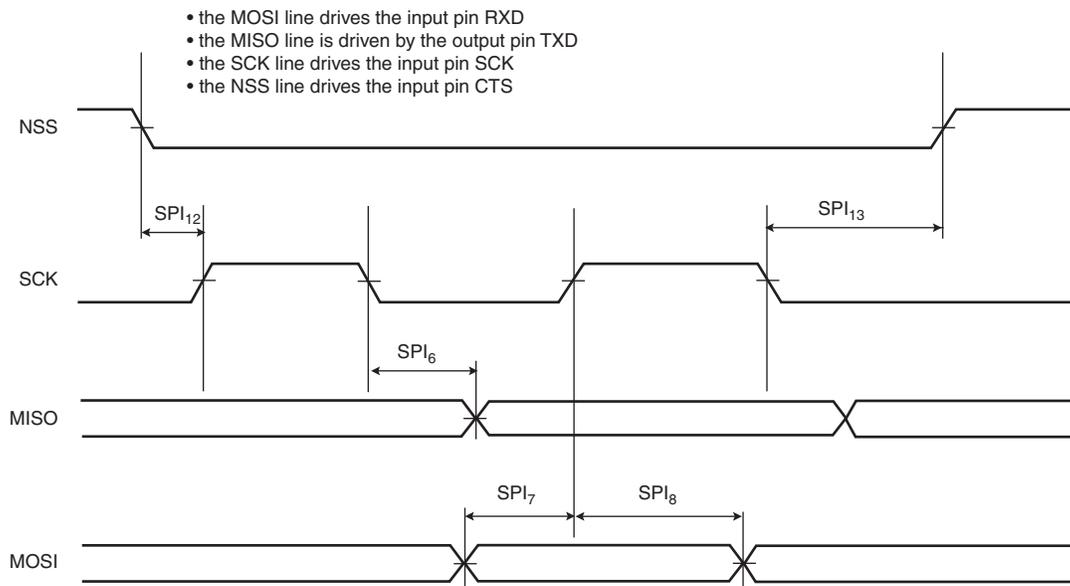
Figure 46-12: USART SPI Slave Mode: (Mode 0 or 3)
