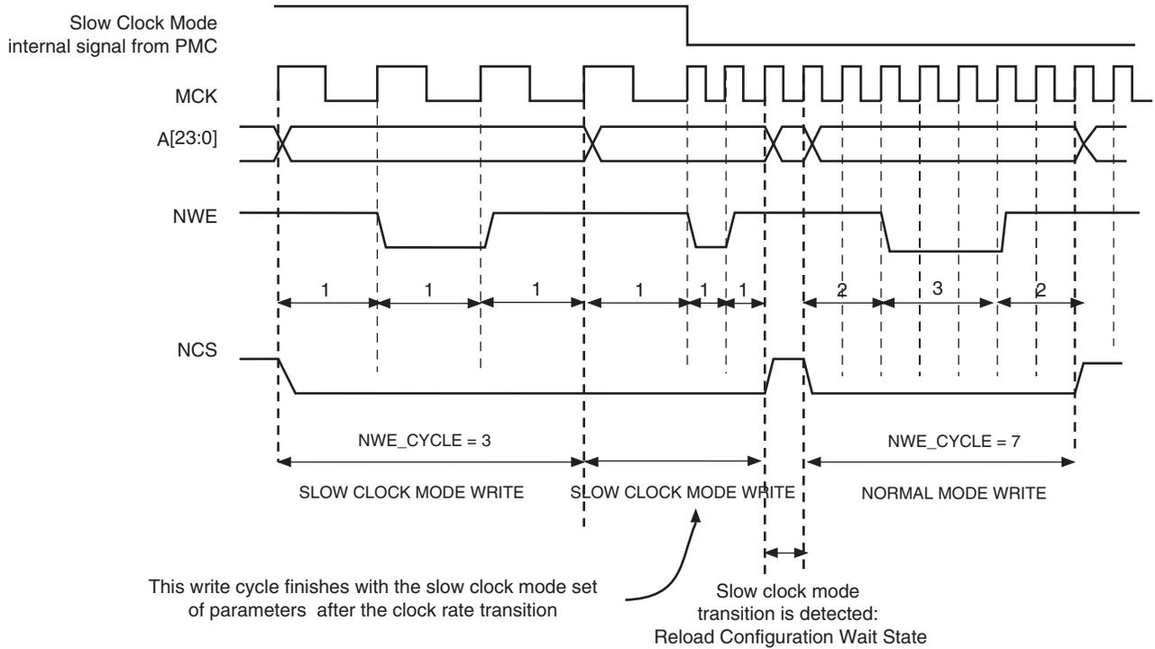
**Figure 27-32: Recommended Procedure to Switch from Slow Clock Mode to Normal Mode or from Normal Mode to Slow Clock Mode**
