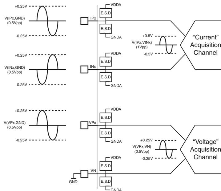
Voltage channels have single-ended inputs referred to the VN pin. This pin must be connected to a low noise ground. The user must take care that no voltage drop on the ground net is sampled by the ADC by non-optimum connection of the VN pin.
