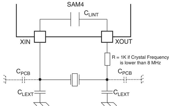
$$C_{LEXT} = 2 \times (C_{CRYSTAL} - C_{LINT} - C_{PCB} / 2).$$
