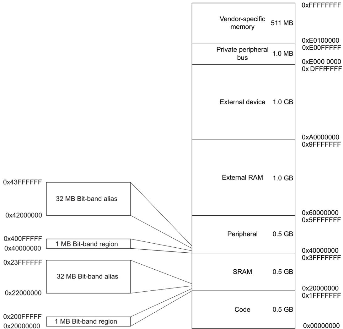
The regions for SRAM and peripherals include bit-band regions. Bit-banding provides atomic operations to bit data, see [“Bit-banding”](#). The processor reserves regions of the *Private peripheral bus* (PPB) address range for core peripheral registers. This memory mapping is generic to ARM Cortex-M4 products. To get the specific memory mapping of this product, refer to [Section 8. “Memories”](#).
