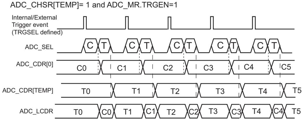
Notes: ADC\_SEL: Command to the ADC cell
