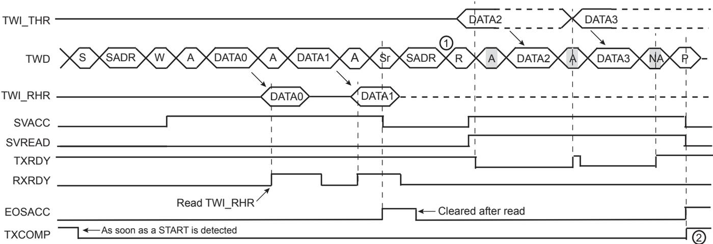
**Note 1:** In this case, if TWI\_THR has not been written at the end of the read command, the clock is automatically stretched before the ACK.
