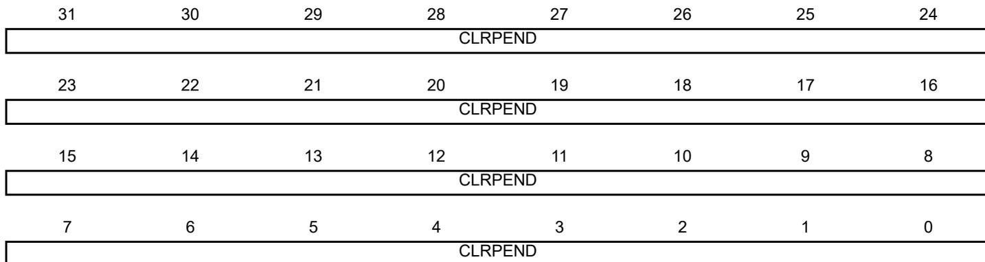
These registers remove the pending state from interrupts, and show which interrupts are pending.
