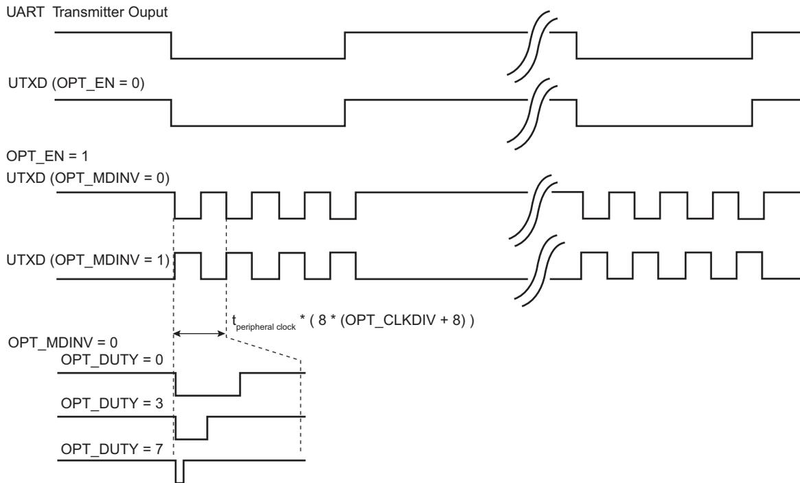
The default configuration values of the optical link circuitries allow the 38 kHz modulation, a 50% duty cycle and an idle polarity allowing a direct drive of an IR LED through a resistor (see [Figure 35-13](#)).
