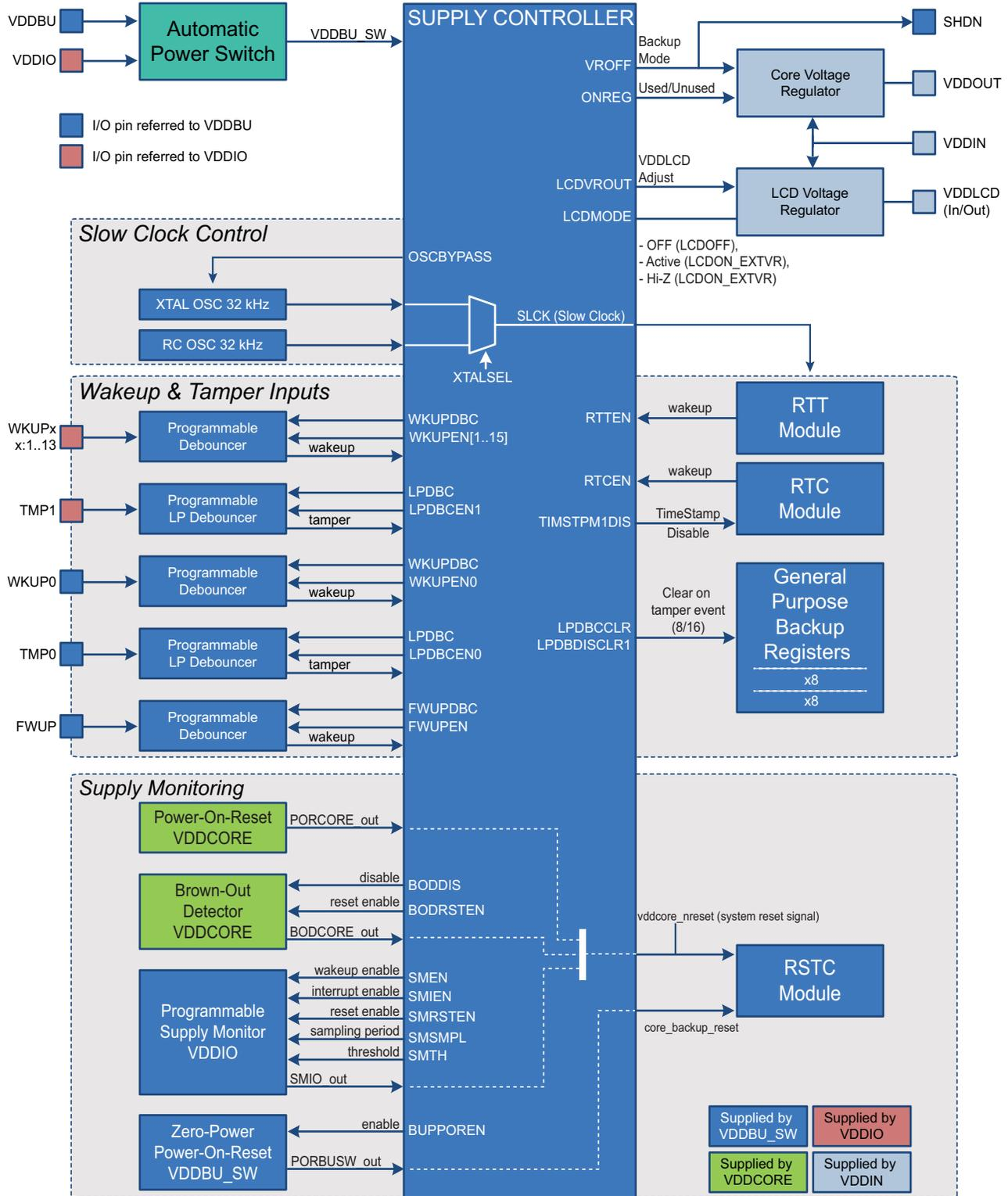
Note: TMPx signals and WKUPx signals are multiplexed on the same pins (e.g., TMP0/WKUP0, TMP1/WKUP10, etc.). This generates a wakeup event only, a tamper event only or a wakeup and a tamper event.
