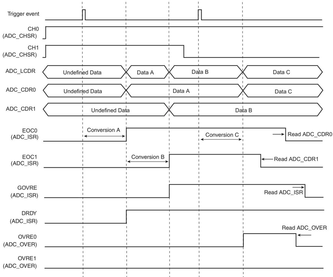
**Warning:** If the corresponding channel is disabled during a conversion or if it is disabled and then reenabled during a conversion, the associated data and the corresponding EOCx and GOVRE flags in ADC\_ISR and OVREx flags in ADC\_OVER are unpredictable.
