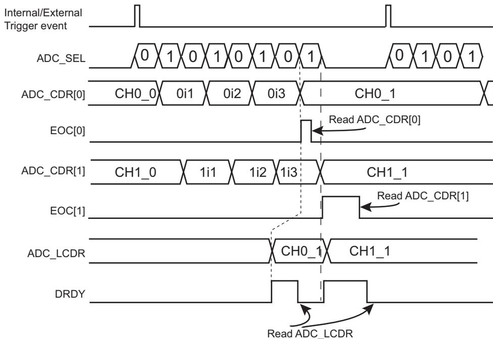
Notes: ADC\_SEL: Command to the ADC cell
