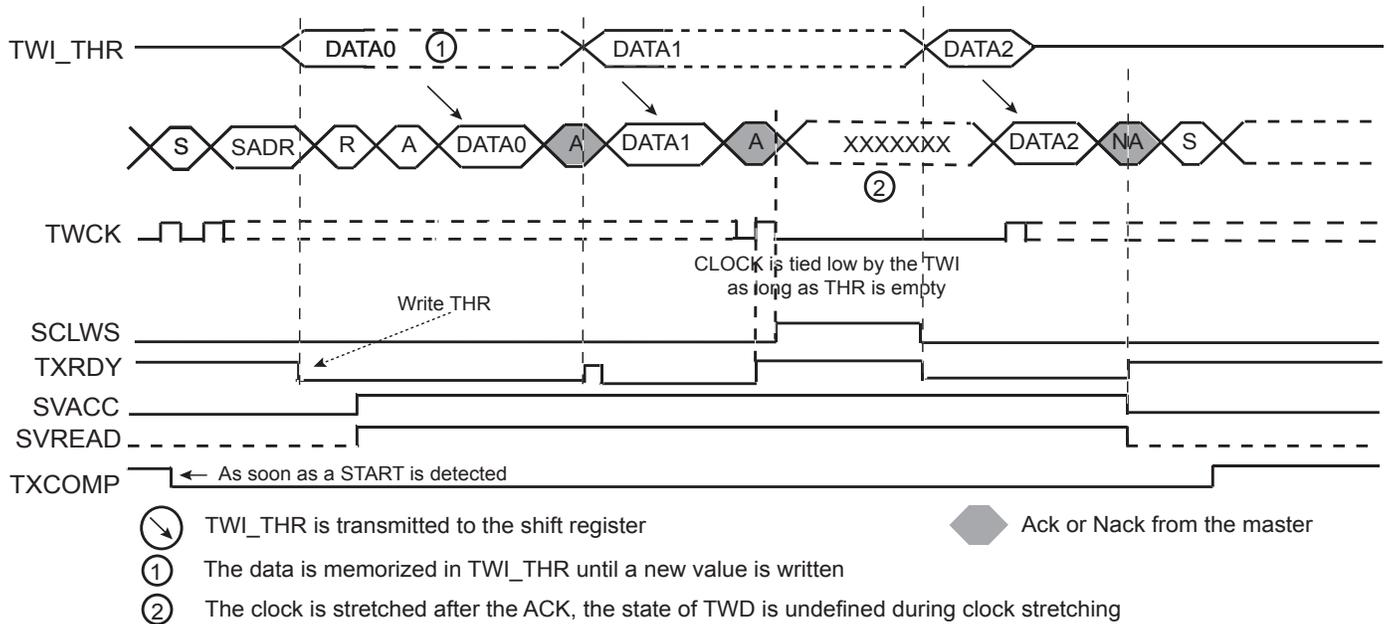
**Note 1:** TXRDY is reset when data has been written in the TWI\_THR to the internal shifter and set when this data has been acknowledged or non acknowledged.
