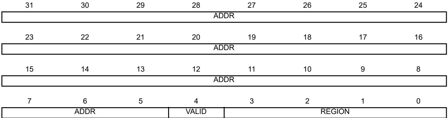
The MPU\_RBAR defines the base address of the MPU region selected by the MPU\_RNR, and can update the value of the MPU\_RNR. Write MPU\_RBAR with the VALID bit set to 1 to change the current region number and update the MPU\_RNR.
