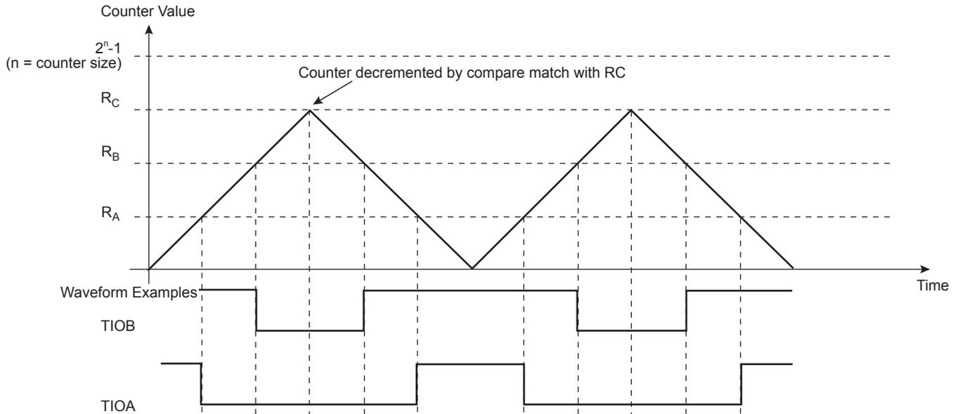
**Figure 37-14: WAVSEL = 11 with Trigger**
