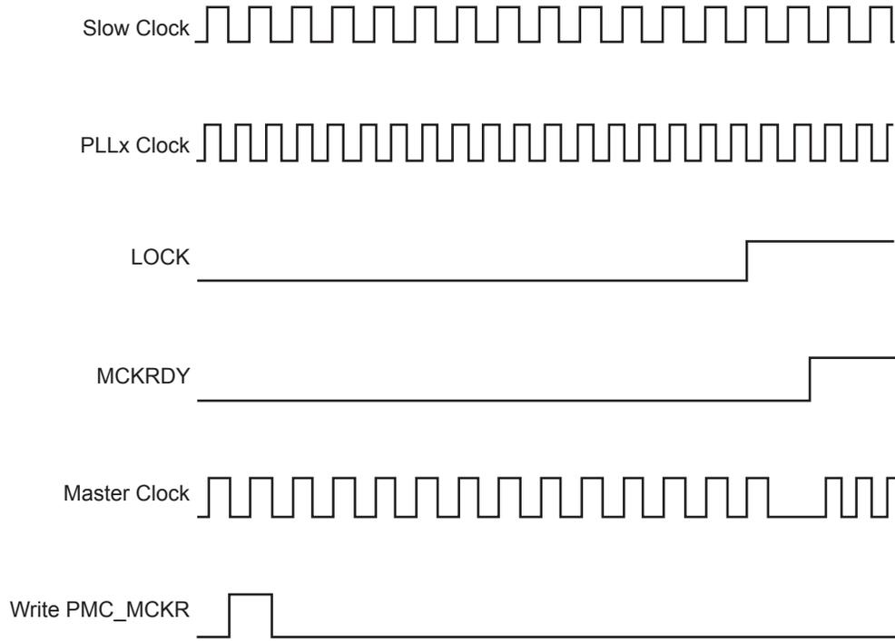
**Figure 30-8: Switch Master Clock from Main Clock to Slow Clock**
