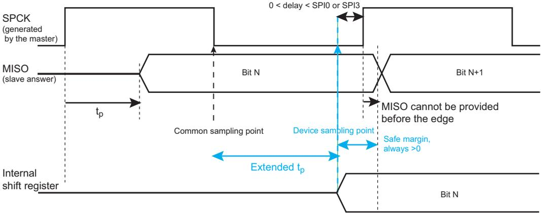
**Figure 46-4: SPI Master Mode with (CPOL= NCPHA = 0) or (CPOL= NCPHA= 1)**
