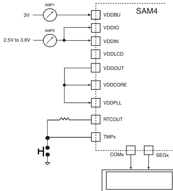
**Note:** No current is drawn on VDDIN power input in Backup mode. The pin VDDIN can be left unpowered in Backup mode.
