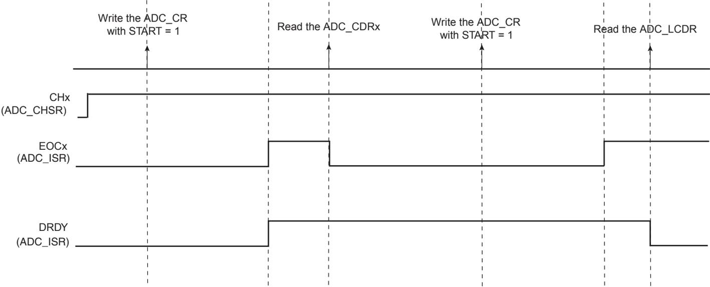
If ADC\_CDR is not read before further incoming data is converted, the corresponding Overrun Error (OVREx) flag is set in the Overrun Status register (ADC\_OVER).
