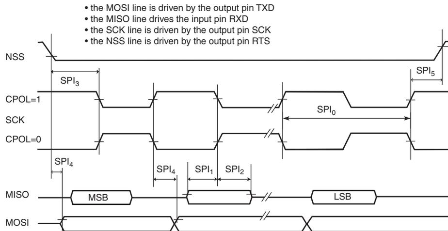
**Figure 46-11: USART SPI Slave Mode: (Mode 1 or 2)**
