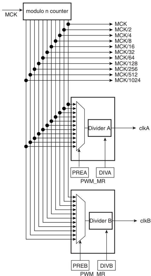
**Caution:** Before using the PWM macrocell, the programmer must first enable the PWM clock in the Power Management Controller (PMC). The PWM macrocell master clock, MCK, is divided in the clock generator module to provide different clocks available for all channels. Each channel can independently select one of the divided clocks.
