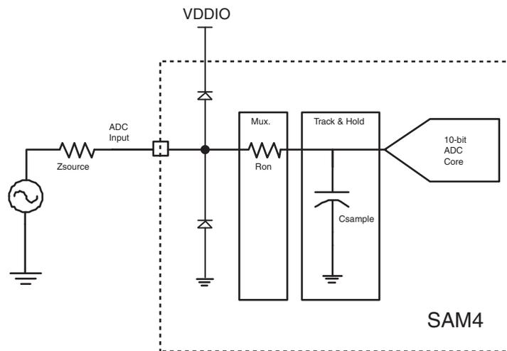
During its tracking phase, the 10-bit ADC charges its sampling capacitor through various series resistors: source output resistor, multiplexer series resistor and the sampling switch series resistor. In case of high output source resistance (low power resistive divider, for example), the track time must be increased to ensure full settling of the sampling capacitor voltage. The following formulas give the minimum track time that guarantees a 10-bit accurate settling:
