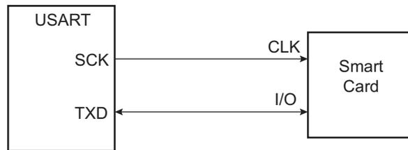
When operating in ISO7816, either in T = 0 or T = 1 modes, the character format is fixed. The configuration is 8 data bits, even parity and 1 or 2 stop bits, regardless of the values programmed in the CHRL, MODE9, PAR and CHMODE fields. MSBF can be used to transmit LSB or MSB first. Parity Bit (PAR) can be used to transmit in normal or inverse mode. Refer to [Section 36.7.3 "USART Mode Register"](#) and ["PAR: Parity Type"](#).
