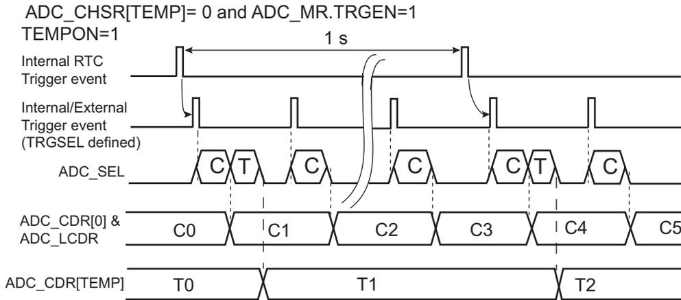
Notes: ADC\_SEL: Command to the ADC cell
