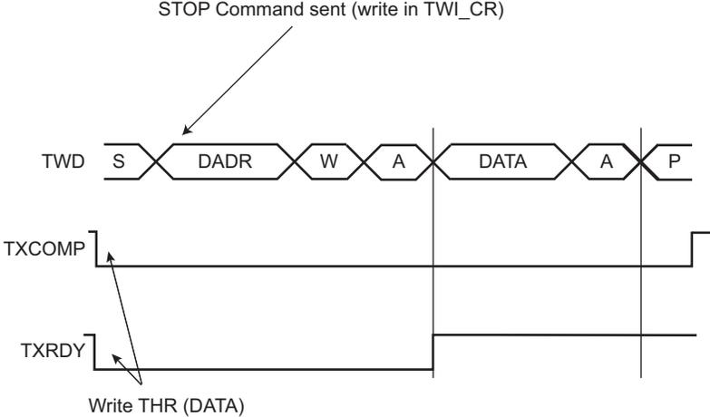
**Figure 34-6: Master Write with Multiple Data Bytes**
