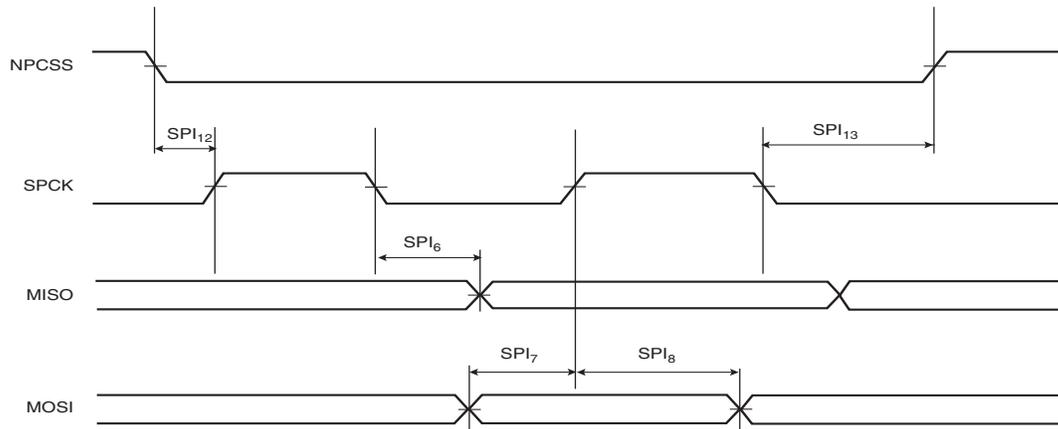
Figure 46-7: SPI Slave Mode with (CPOL = NCPHA = 0) or (CPOL= NCPHA= 1)
