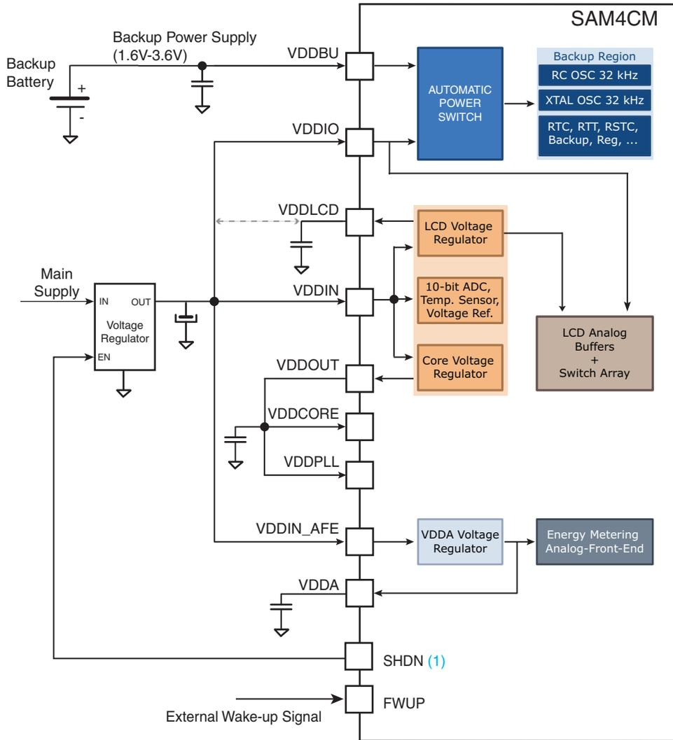
**Note 1:** Example with the SHDN pin used to control the main regulator enable pin. SHDN defaults to VDDBU at startup and when the device wakes up from a wake-up event (external pin, RTC alarm, etc.). When the device is in Backup mode, SHDN defaults to 0.
