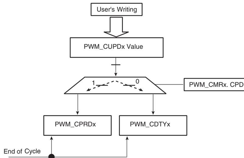
To prevent overwriting the PWM\_CUPDx by software, the user can use status events in order to synchronize his software. Two methods are possible. In both, the user must enable the dedicated interrupt in PWM\_IER at PWM Controller level.
