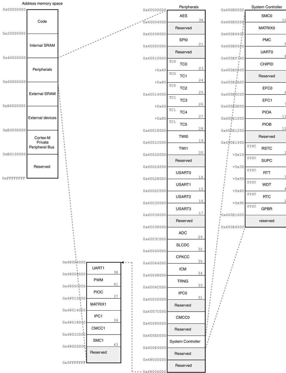
**Figure 7-6: SAM4CM32/16/8/4 Memory Mapping of External SRAM and External Devices Area**
