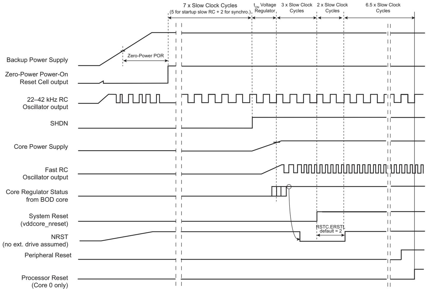
Note: After processor reset rising, the core starts fetching instructions from Flash at 4 MHz.
