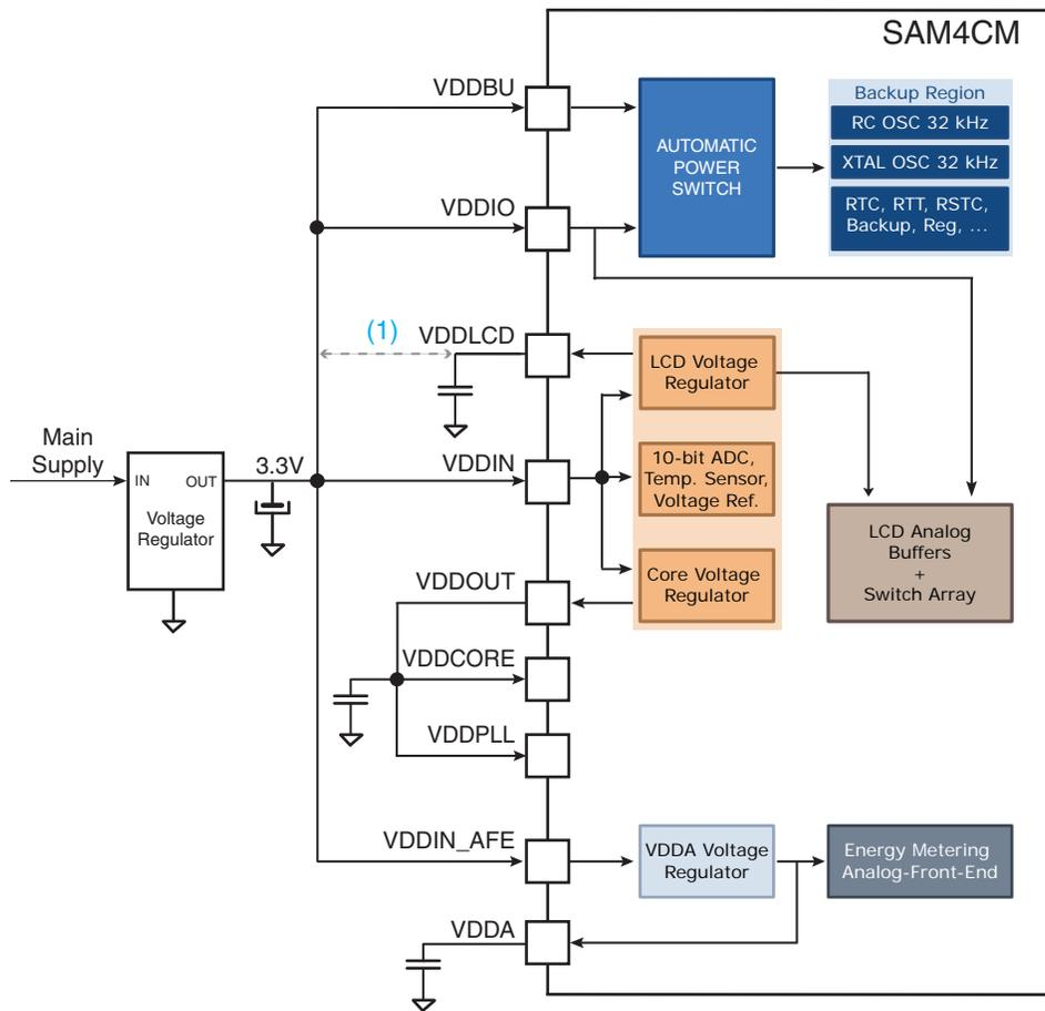
**Note 1:** Internal LCD Voltage Regulator can be disabled to save its operating current. VDDLCD must then be provided externally.
