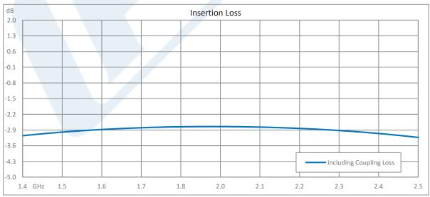
Click the following link (or enter part number in "SEARCH" on website) to obtain additional part information including price, inventory and certifications: 90 Degree SMA Hybrid Coupler from 1.4 GHz to 2.5 GHz Rated to 50 Watts PE2CP1145
